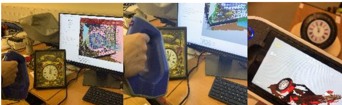
Figure 4: Left clock digitization process. In the background you can see a part of the model on the monitor which is also captured with the texture. If the software throws up an error then entire image must be recalculated. It is then possible to continue digitizing. The image on the right is the digitization process with the Artec Leo scanner. The scanner has a small display so it is necessary to connect it to the computer only in the case of data transfer to the Artec Studio program, in which the resulting 3D model will be modified and created
